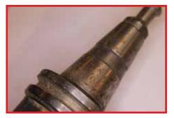
1. Check tools for any debris or rust on the surface of the tool holder
