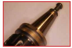
3. Surface should be smooth and clean to prevent damaging the spindle.
