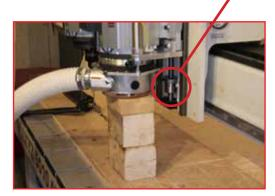
3. Support the Z - plate and tool with a sturdy platform.
