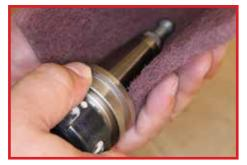
2. Use a cleaning pad or steel wool to clean the tool holder ( do not use sand paper or a file)
