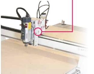
**Oil Oscillating Knife:** Oil the oscillating knife (1-2 drops, every 4 hours).
